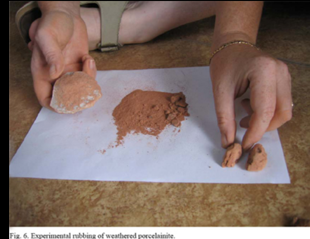
Fig. 6. Experimental rubbing of weathered porcelainite.
